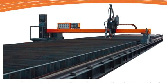
The range of cutting tables Plasmacut Powerful are modular machines with movable bridge and independent fixed table for heavy loads, with convertible frame for submerged cutting areas and selectorized suction system for dust and fumes.
